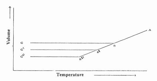
Fig.(1.2): The relation between the volume and temperature for a glass of the same composition but with different densities.
