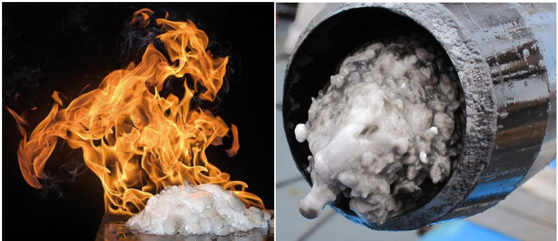
Figure-2: Gas hydrate recovered from piston corer at 2550 m water (Helen Gibbons, 2010).
