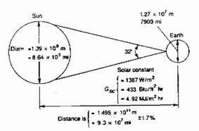
Fig. 1-2: The geometry of the sun-earth relationship.
