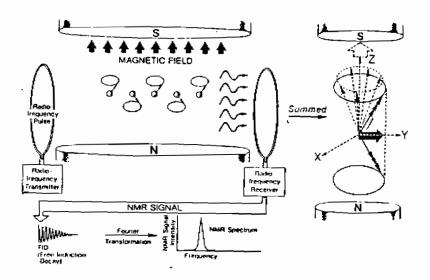
Fig. (1-5): Shows the RF transmitter, RF receiver, where the signal passes through a fourier transformer and signal production (Harms et al., 1984).
