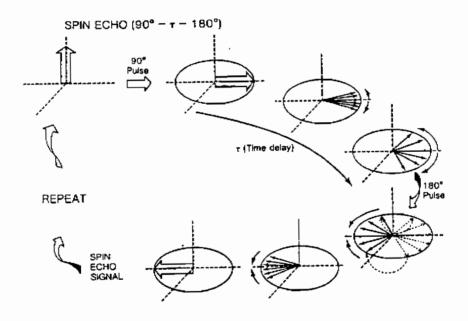
Fig. (1-6): Showing the SE pulse sequence (Harms et al., 1984).
