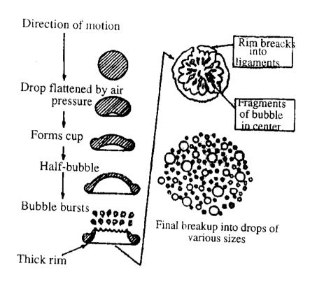
Fig. 2.1: Breakup of a spherical drop by interaction with ambient air (lefebfre, A.H. 1989).
