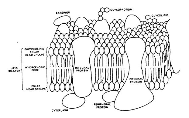
Fig. 1: Model of membrane structure. The continuous double layer of phospholipid molecules is arranged with polar headgroups at the membrane surface and the fatty acid chains meeting in the interior of the membrane. Integral proteins are embedded in the bilayer whereas peripheral proteins are loosly attached at the membrane surface. Carbohydrates group are confined exclusively to the external or normocytoplasmic membrane surface.
