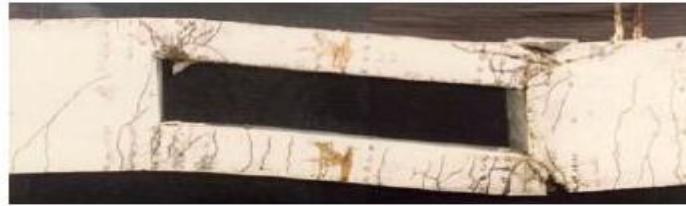
Figure (2.12) Ductile failure of a beam under combined bending and shear, (Mansur et al. , 2001) [13]
