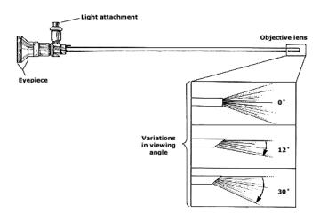
Fig. (1): Hysteroscope with different viewing angles (Guido, 2006).
