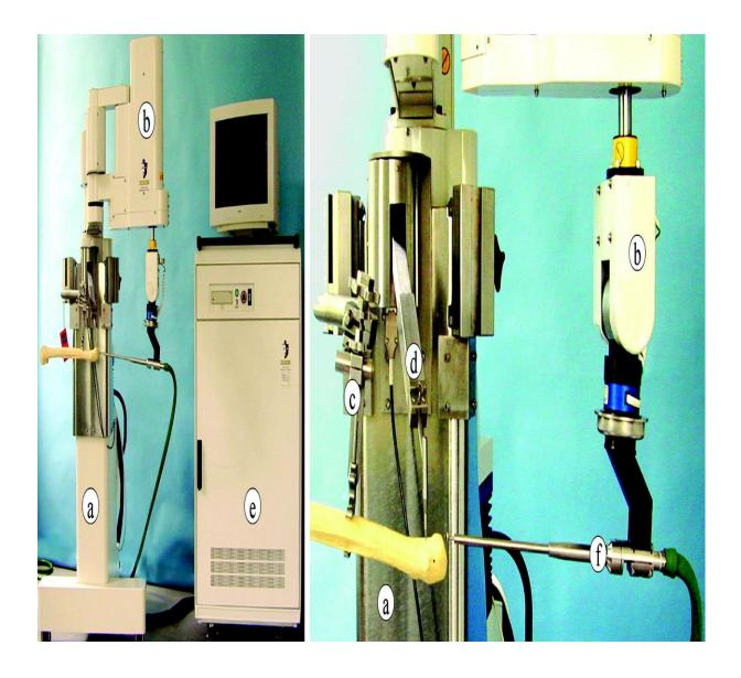
**Fig.** (1) The ROBODOC surgical robot. a = robot base, b = robot arm with  $5^{\circ}$  of freedom, c = the femoral fixator, d = the bone-motion detector, e = the control computer, and f = the pneumatic turbine with the reamer bearing sleeve. [5]
