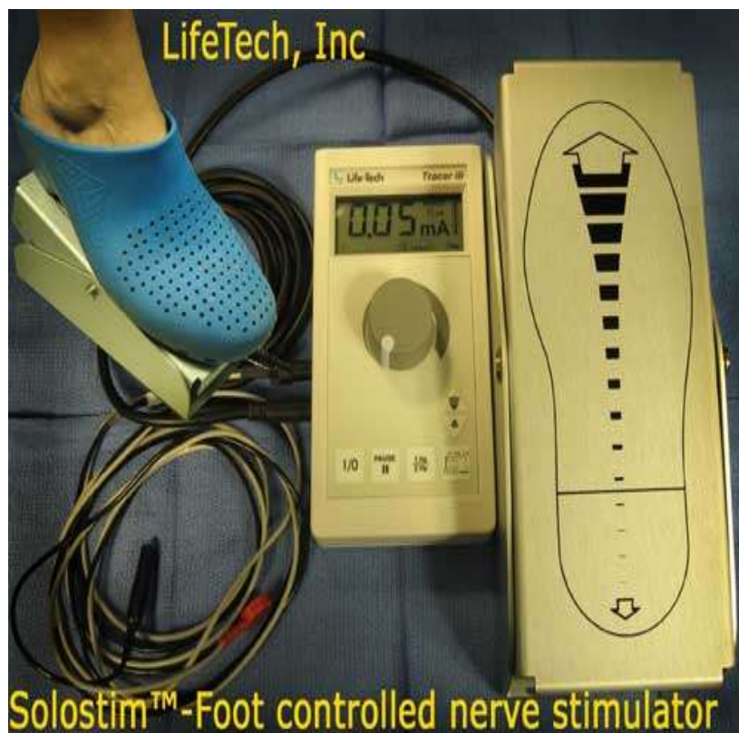
Fig(2) Foot controlled nerve stimulator ( New york school of regional anesthesia ).
