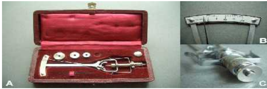
Fig. (1): Schiøtz indentation tonometer. A = Case, B = Scale, C = Concave foot with central plunger ( Kniestedt, 2008 ).
