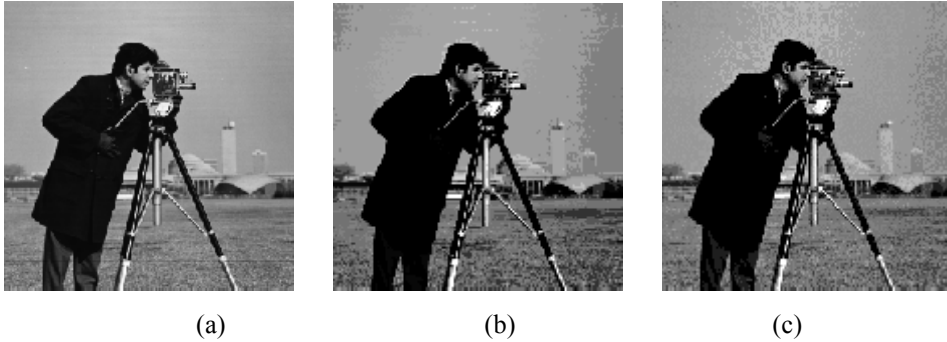
Figure 1.1: Uniform vs IGS quantization. (a) The Original Image; (b) Uniform quantization to 16 levels; (c) IGS quantization to 16 levels.
