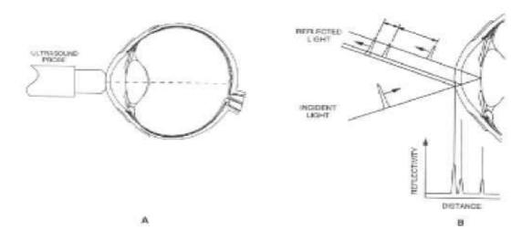
Figure (1): Ultrasound axial measurement (A-mode) and imaging (B- mode) require direct contact with the eye (A), while optical axial imaging have higher resolution than ultrasound and do not require direct contact with the eye (B). [19].
