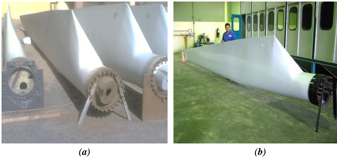
Figure 1-1 (a) The original blade (Ventis) and (b) The manufactured blade locally
