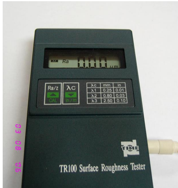
Fig. (^) TIME surface roughness tester
