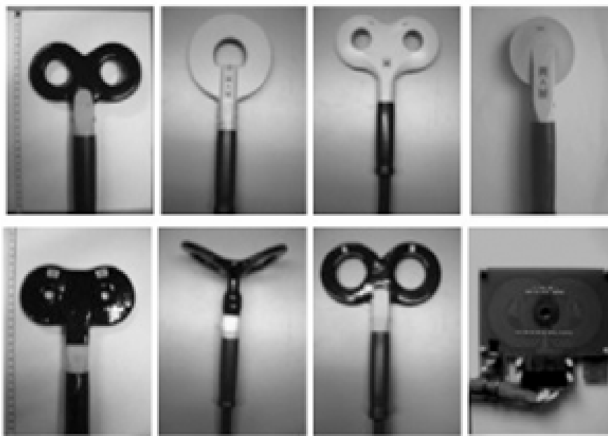
Figure (2): Different stimulation coils used for TMS interventions which differ in field shape, size and depth: (first line left to right); 40-mm diameter figure-of-eight, butterfly or double coil, 70-mm circular coil, 70-mm butterfly coil, 50-mm circular coil; (second line) 45-mm butterfly coil, bell-shaped coil, 50-mm butterfly coil, 50-mm butterfly coil with an integrated 0.7-mm thick heat-resistant card to be used in combination with intracranial recordings in animal models ( Valero-Cabré et al., 2017 ).
