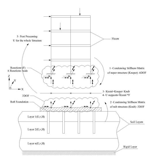
Figure 1.1 The proposed new method of static condensation.
