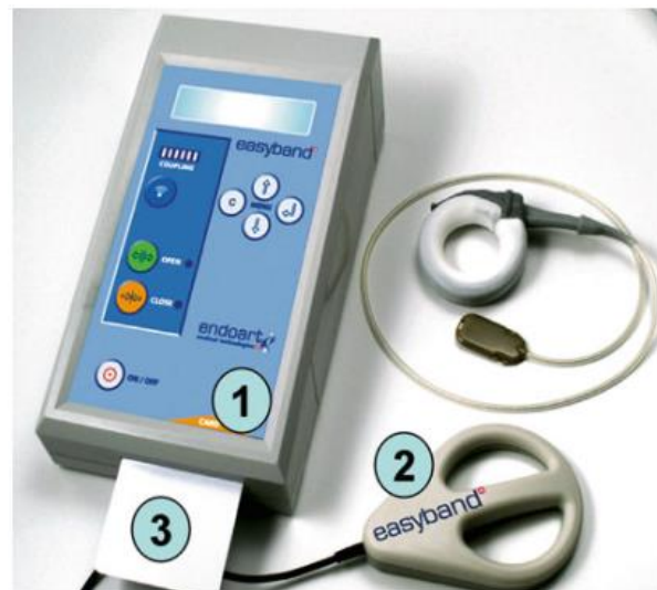
Figure (3): Remote adjustable Gastric band (courtesy of Allergan). (1) A control unit sends energy and information telemetrically to the easyband through magnetic induction. (2) Antenna: magnetic induction is sent to the antenna, which is connected to the easyband. (3) A microchip saves the adjustments of the easyband ( Korenkov et al., 2012 ).
