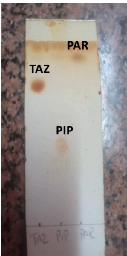
Fig. 4. TLC plate showing separation of tazobactam (TAZ, 400 \mu\text{g}/\text{band} ), piperacillin (PIP, 60 \mu\text{g}/\text{band} ), and paracetamol (PAR, 80 \mu\text{g}/\text{band} ) after iodine vapor visualization.
